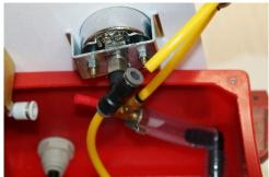
5. Using an 11/16 wrench, loosen and remove the plastic hose barb. Once removed, you can pull out the entire venturi assembly, as shown below.
