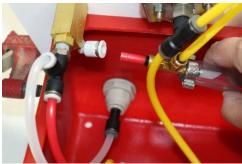
4. Follow the ½ yellow tubing connected to the venturi until you reach the Adapter Tee. Remove the yellow tubing from the push to connect tee, on the back of the gauge, as shown below.
