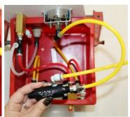
3. The yellow tube from the 90 degree elbow will be re-installed into the plastic push to connect fitting shown below.
