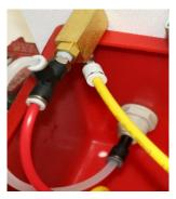
4. Slip the Teflon gasket over the threads on the venturi and slip the venturi into the hole at the bottom of the control console. The metal washer will then be installed over the threads followed by the plastic bulkhead, as shown below. Tighten down the bulkhead.
